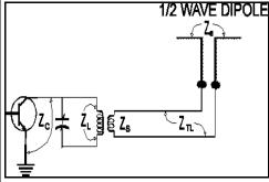
The impedance of the antenna Z<sub>a</sub> (70 a 500 Ohm load will present a mismatch, Ohms) must match the *surge impedance* of the two wire transmission line,  $Z_{TL}$ . The impedance of secondary of the output transformer, Z<sub>s</sub>, which must couple tight enough to reflect an impedance across the primary,  $Z_L$ , that must match the collector impedance of the transistor Z<sub>c</sub>. A variation of any part of this chain may prevent maximum output.
